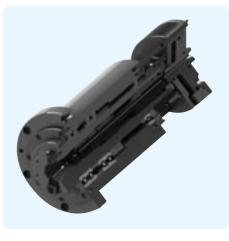
Example of spindle unit specification Machine used Machining center Mounting orientation Vertical Rotational Speed Max. 10,000 rpm (Max. 700 rpm without tooling attached) Spindle taper size #30 Lubrication methods Grease lubrication Lubricant ISOFLEX NBU15 (NOK Corporation) Tool clamping power 400 kgf (theoretical) 3.5kW Estimated drive power Estimated weight 31kg
